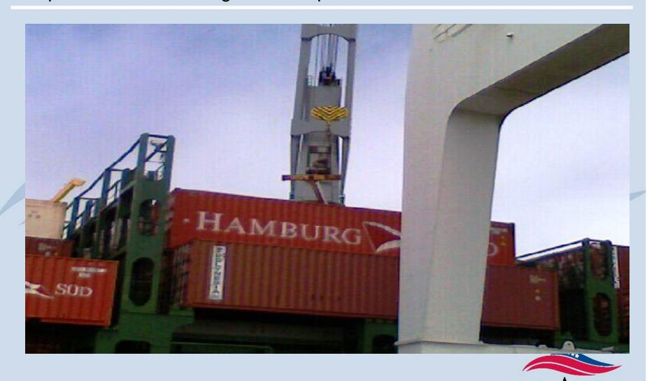
The Dock crane was in the boomed up position while gantrying aft. Collision sensors on the shore crane are not active in the boomed up position.
